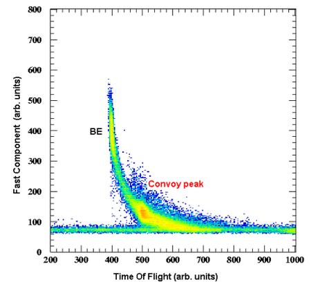
A typical fast-slow component bidimensional plot to charge identify the nuclear products for the reaction  $^{40}\text{Ar} (77 \text{ A.MeV}) + ^{27}\text{Al}$ .
