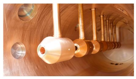
In Sweden, at the ESS, *European Spallation Source*, research centre which will host the world's most powerful neutron source in Lund, the first protons passed through the Drift Tube Linac 1, DTL1, one of the key components of the ESS accelerator built in Italy by INFN researchers.
